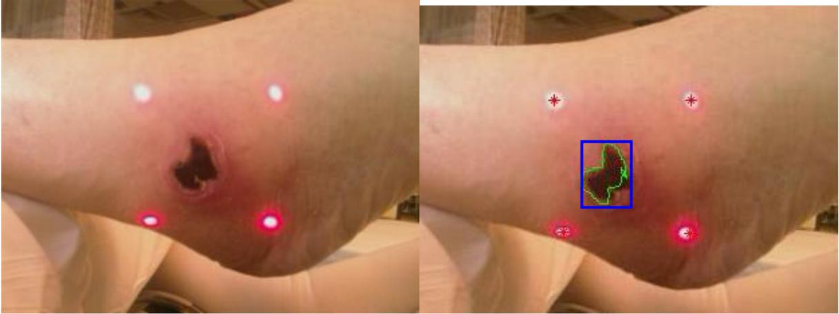
Figure 12. Original image is on the left. The processed image with lasers identified (red stars), border drawn (green), and ruler-based rectangle (blue) is on the right.
