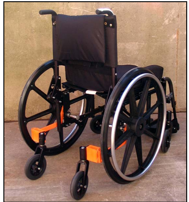
Folding K0001 with rear casters and pivot arms.
