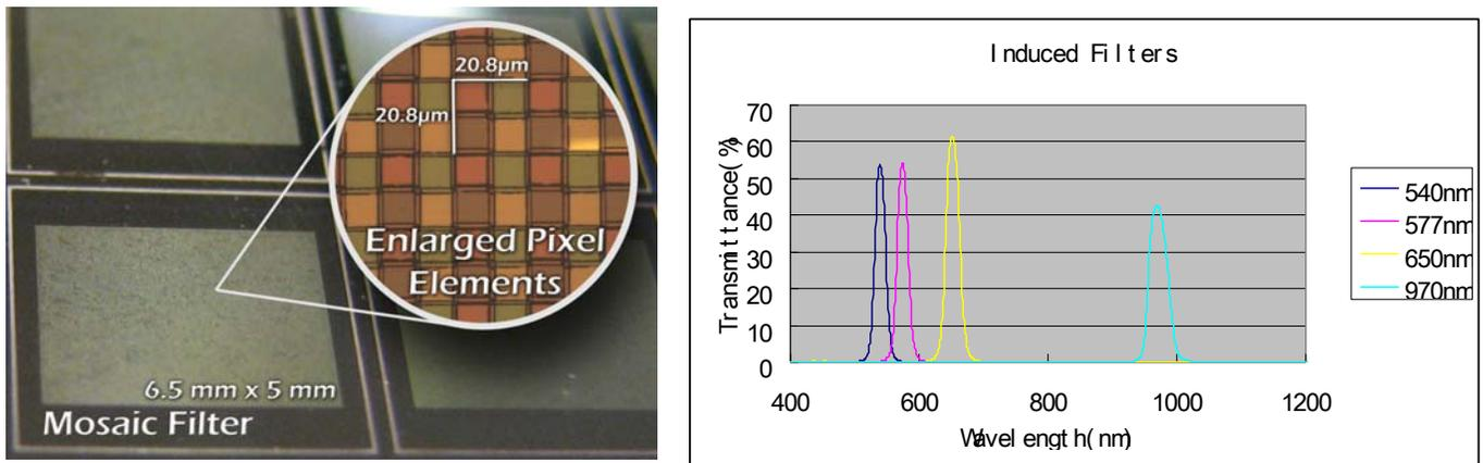
**illumination system.** One challenge in creating a clinical multispectral instrument is the variable ambient lighting conditions. For the mosaic filter to work properly, the clinical target must be bathed in light that contains the spectra of interest. In addition, lighting requirements must be compatible with the portability requirements of a handheld device. Specifically, we desired a battery-operated device that can be carried in a lab coat, so size and weight were important considerations.
