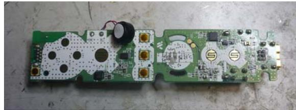
Figure 2: Wiimote Circuit Board
