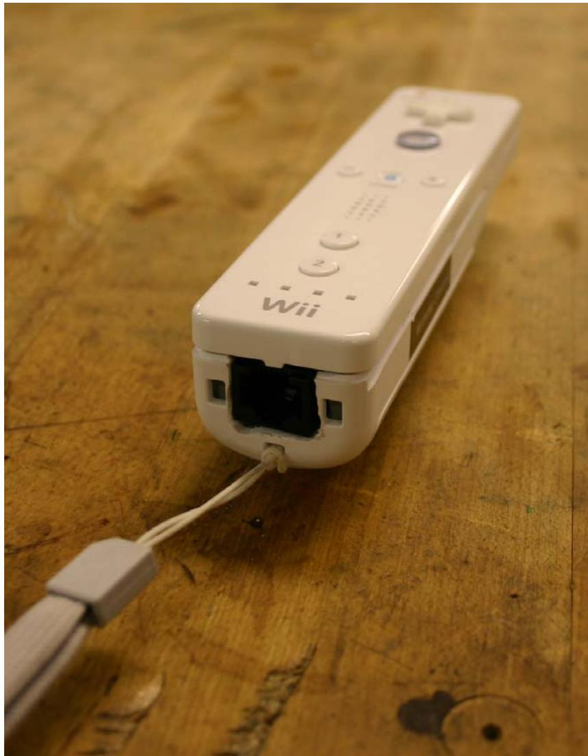
Figure 17: Completed Wiimote with 8P8C Ethernet Port
