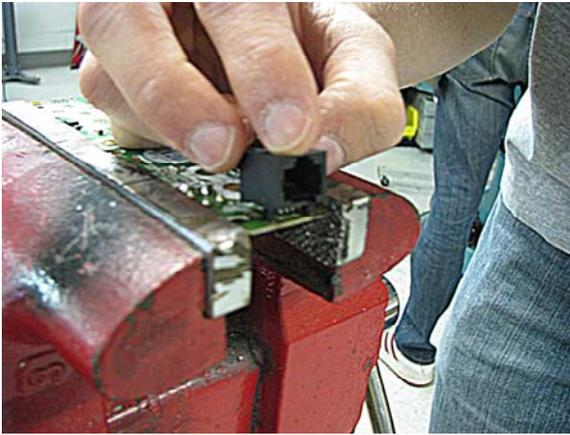
Figure 6: Lining Up of 8P8C Female Port
